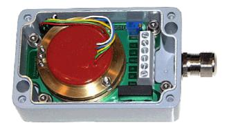
Sensor box containing one highly sensitive servo inclinometer and one signal conditioner with ±5V output
